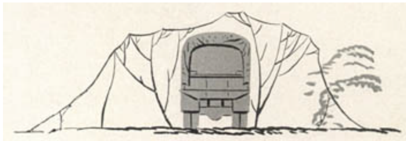
FIGURE 46 (1). Nets must be propped above and away from a vehicle so that a distorted outline is formed. Branches or poles are used for this purpose. To eliminate shadow, extend net at a gradual slope from centre of object covered.
